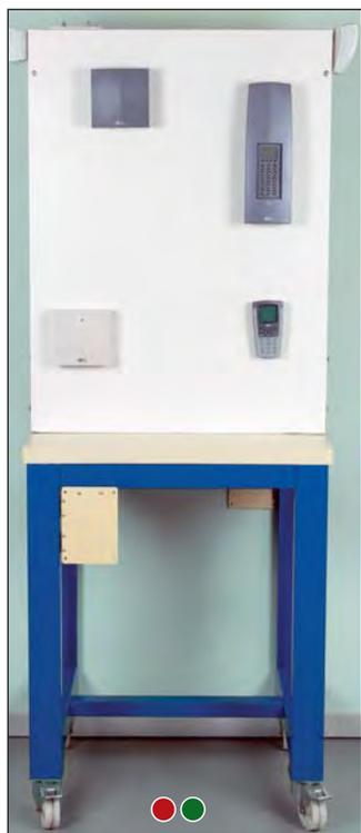
GES-7 is a programming and wiring panel for a BUS wired (two wires) anti-intrusion alarm unit. This unit monitors two areas in the business premises by means of a passive infrared sensor, a dual-technology intrusion sensor (infrared + microwave frequency) and two magnetic sensors which are triggered if the windows are opened. A keypad for entry code, which is built into the unit, activates or deactivates monitoring of the area.
