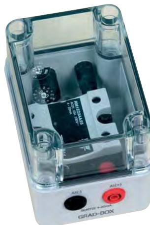
Controls the power in the charge by varying the conduction angle of the thyristors according to the control current of 4-20mA. Can be connected directly to the built-in PLC unit ref. AUTO-BOX-A.
