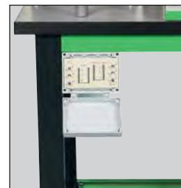
Unit with concealed switches to simulate sensor faults. 6 switches linked to 6 sensors. Unit fixed onto the system's frame.
