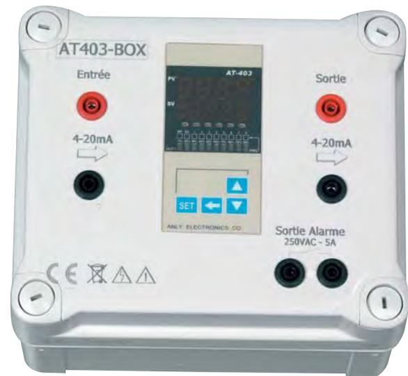
The PID regulator is the correcting component into a regulation loop for the monitoring of a process (boiler, compressor, pump ...). It receives a 4-20mA signal from the sensor which is the image of the value to regulate (temperature, pressure, flow...). It compares it to the set-point (programmed in the PID) and drive the process to reduce the difference "process variable / set-point"
