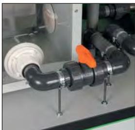
Used to drain the tank, e.g. to simulate reservoir maintenance.
