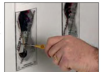
Coupling a receiver + transmitter pair through the protection window by pressing a contact.
