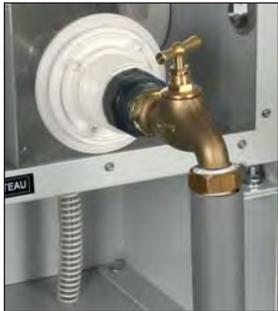
Simulates domestic water consumption. Connected by hoses to the tank that simulates the river.
