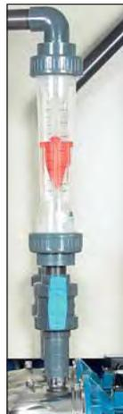
A moving float in a transparent tube indicates the pump's water flowrate in cubic meter/hour
