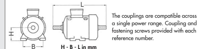
The couplings are compatible across a single power range. Coupling and fastening screws provided with each reference number.
