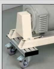
This economical option consists of fixing 4 or 6 castors equipped with brakes directly under the rails. This solution effectively replaces a chair with casters and allows you to easily move your motor unit. This solution raises the assembly by 170mm.
