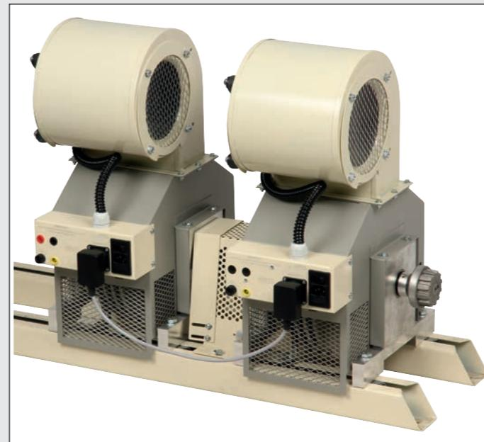
As the powder brakes of the other ranges, a simple DC current under a low voltage around 14V generates a constant braking torque for all the speeds between 0 to 1500 rpm.
