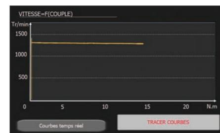
Evolution of speed as a function of torque
