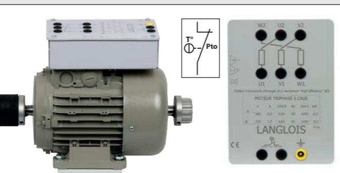
This type of motor works as well on frequency converter as on 50Hz direct mains.
