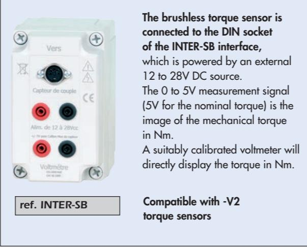
The brushless torque sensor is connected to the DIN socket of the INTER-SB interface, which is powered by an external 12 to 28V DC source. The 0 to 5V measurement signal (5V for the nominal torque) is the image of the mechanical torque in Nm. A suitably calibrated voltmeter will directly display the torque in Nm.
