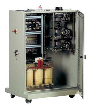
This power supply, which is varied using an autotransformer, can be networked so that it can power other stations. The DC outputs are insulated from the mains, as stipulated in the standard, and monitored by a continuous insulation monitoring device for the safety of users. This monitoring allows the DC output to be networked. The transformer complies with the NFEN6158 norm.
