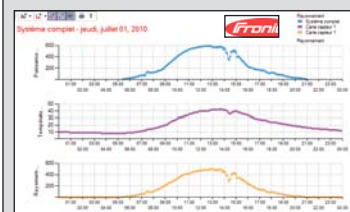
Screenshot of 3 recordings made during the day : Instant alternative power, temperature of panels, intensity of solar radiation.
