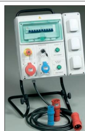
This 460 x 480 x 120mm plastic electrical unit is placed on the ground. It delivers various voltage sources, protected by thermal magnetic circuit breakers. Connection to the 3x400V+N+E electric network via a 5 meters cable and P+E connector. Supplied with plugs for connection to the mains.
