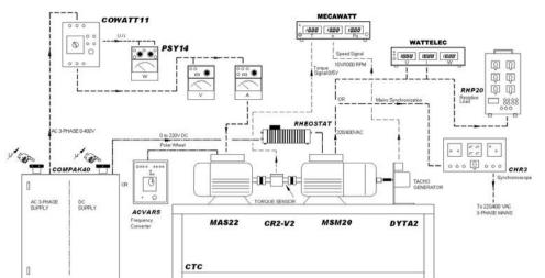
The PACK-AC2 power unit kit (power unit + accessories) can be used for studying a 1500W asynchronous motor.
