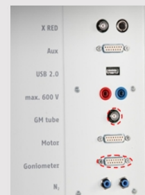
Fig. 3: Connectors in the experiment chamber
