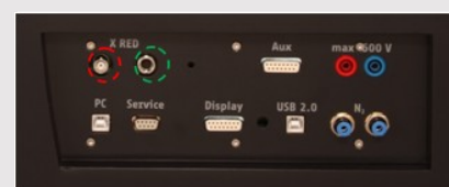
Fig. 4: Connection of the multi-channel analyser
