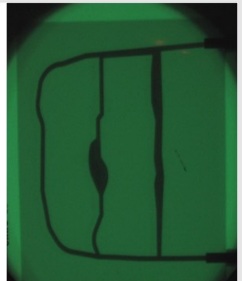
Fig. 1b: Blood vessel model with the contrast medium; completely filled
