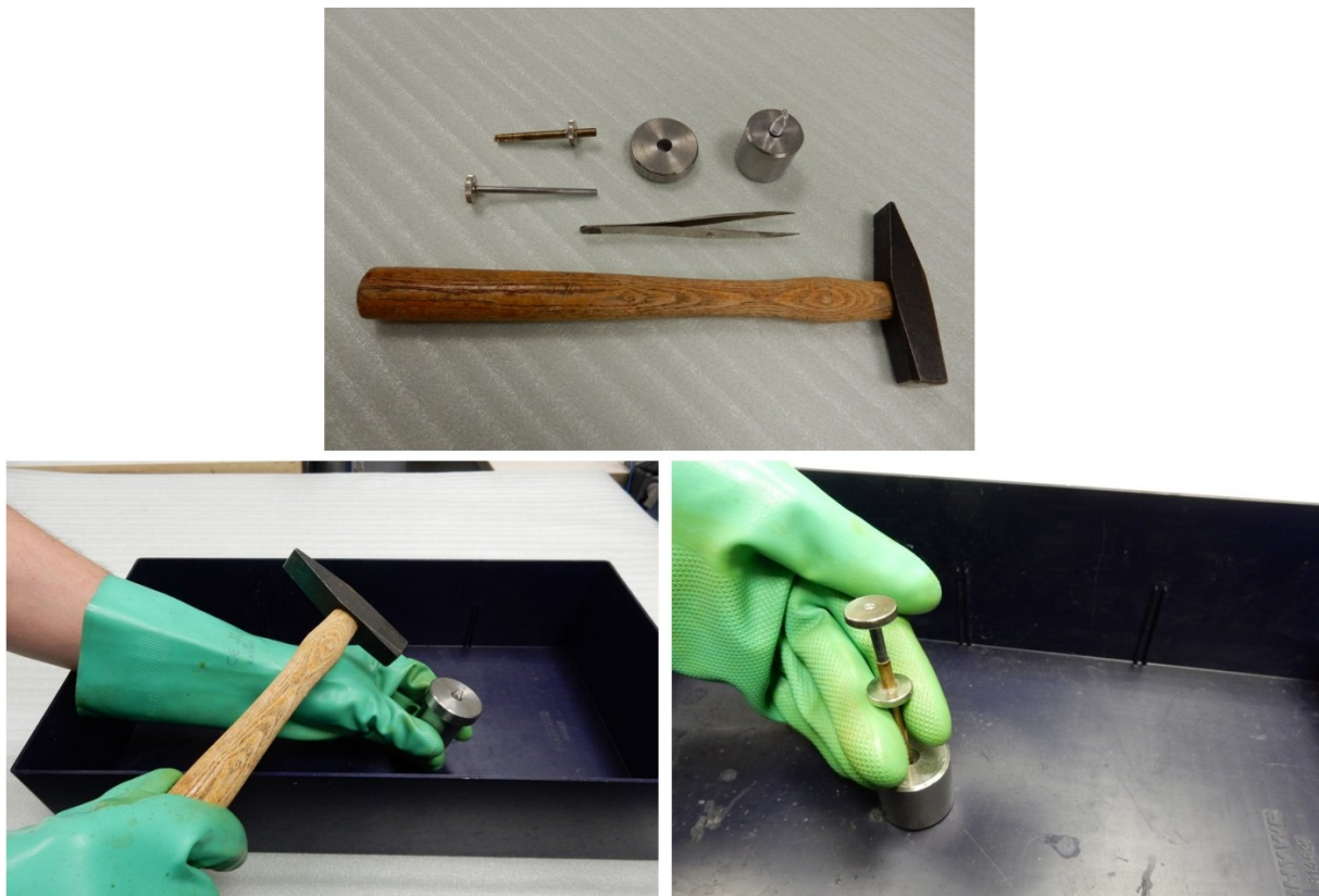
Fig. 2: Breaking the glass ampule in order to load potassium into the furnace.
