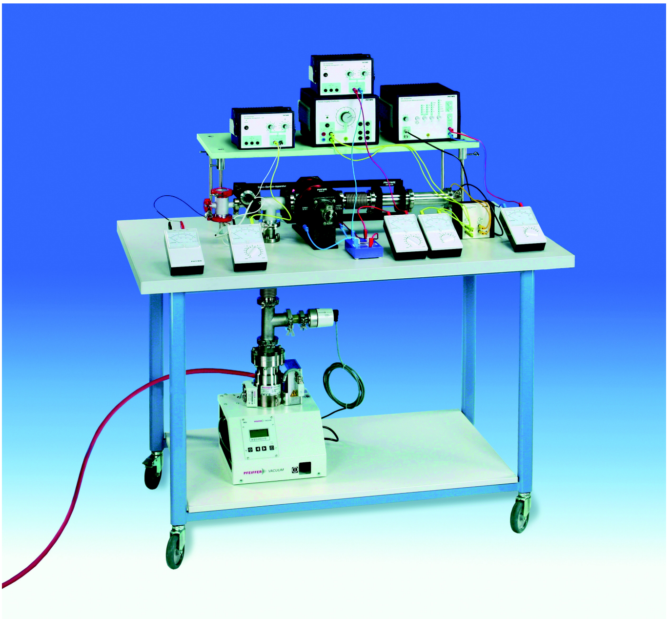
Fig 1: Experimental setup; Stern-Gerlach apparatus with high vacuum pump assembly.
