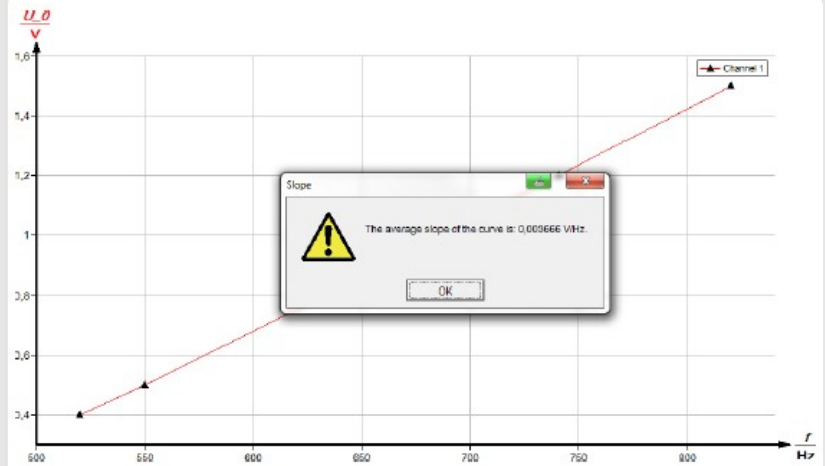
Stopping voltage U_0 as a function of the frequency of the irradiated light
