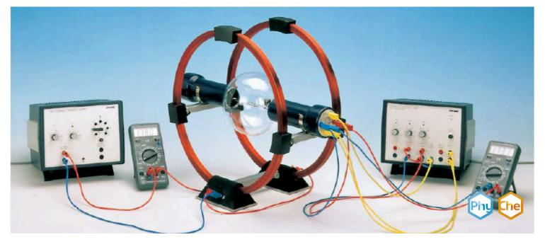
Electrons are accelerated in an electric field and enter a magnetic field at right angles to the direction of motion. The specific charge of the electron is determined from the accelerating voltage, the magnetic field strength and the radius of the electron orbit.
