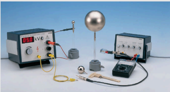
Fig. 1 : Experimental set-up to determine the capacitance of conducting spheres.
