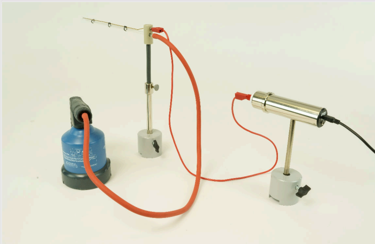
setup for the measurement of the electrical potential
