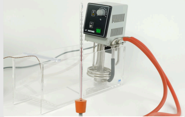
Fig.3. Experimental set-up for measuring thermal expansion
