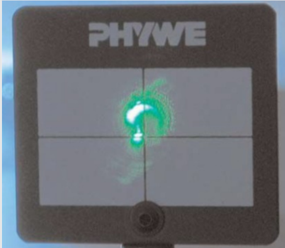
Bad laser tube alignment
