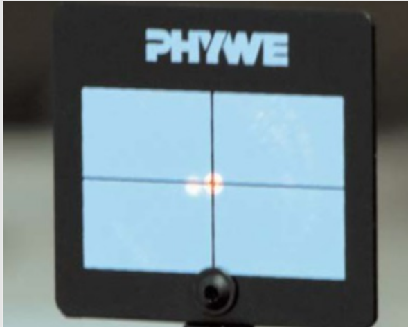
Beam centered on the right diaphragm with ghost beam visible left of it.
