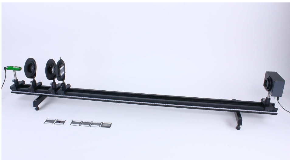
Fig. 1: Experimental set-up to investigate the diffraction intensity of multiple slits and grids.
