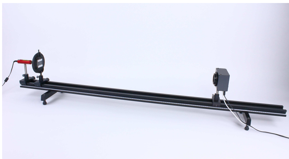
Fig. 1: Experimental set-up to investigate the diffraction intensity of a single slit.
