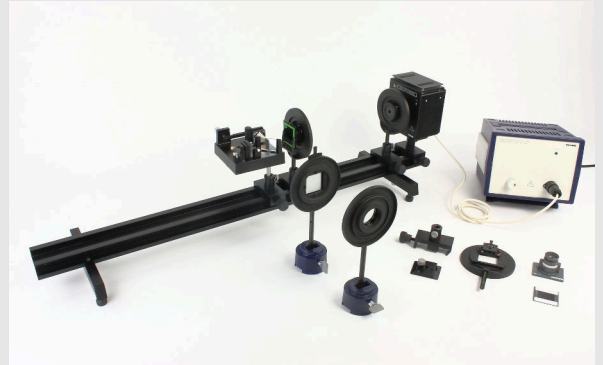
Experimental set-up to determine coherence and wavelength of spectral lines
