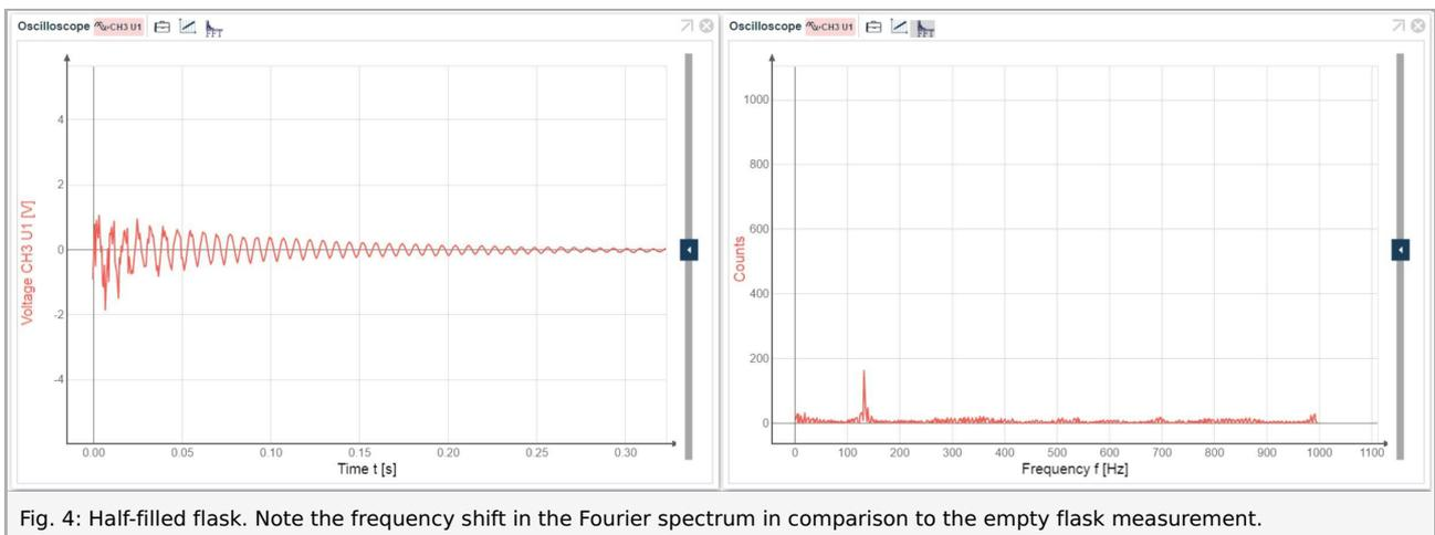
Fig. 4: Half-filled flask. Note the frequency shift in the Fourier spectrum in comparison to the empty flask measurement.
