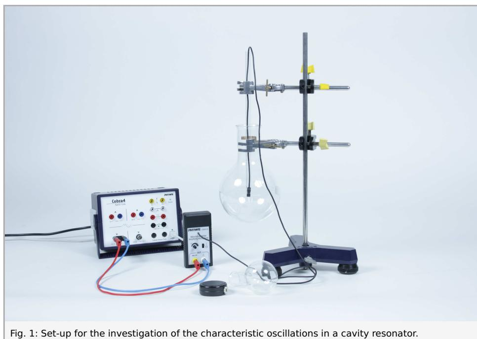
Fig. 1: Set-up for the investigation of the characteristic oscillations in a cavity resonator.
