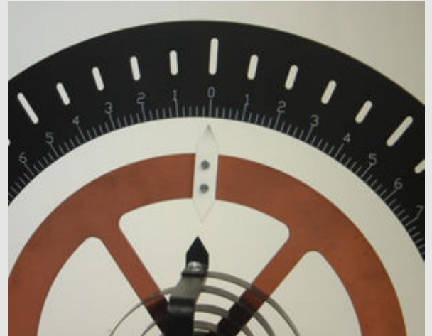
Fig. 4: Pendulum pointer at zero-position.
