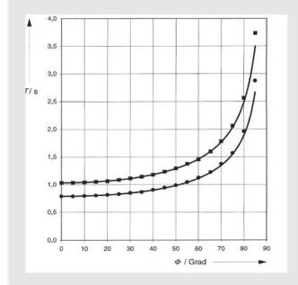
Fig 2: Oscillation period of the pendulum as a function of the slope  $\Phi$  of the oscillation plane. The measured points are plotted above the corresponding theoretical curve(solid line). Upper curve: L = 270 mm; lower curve: L = 141 mm.
