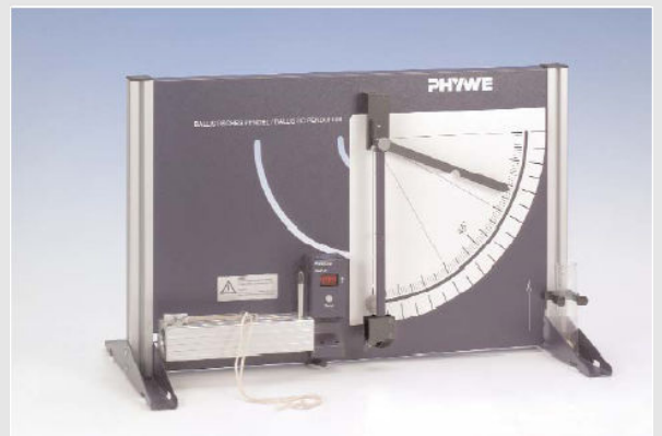
Fig. 3: Experimental set-up with supplement for direct measurement of the initial velocity of the ball.
