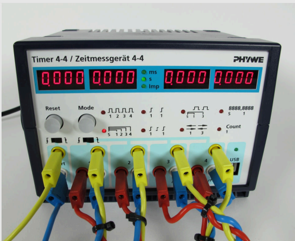
Connecting the light barriers and the starting device
