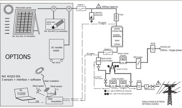
Kit of photovoltaic components for studying a solar installation with total or partial energy injection to the electricity network 230VAC-50Hz.
