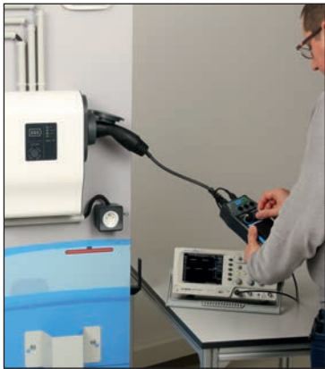
Charging station tester delivered with the model.
