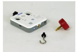
Fig. 11+12 Float and sensor with magnet
