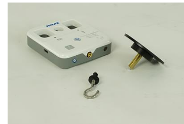
Fig. 7 Sensor with hook and weight plate
