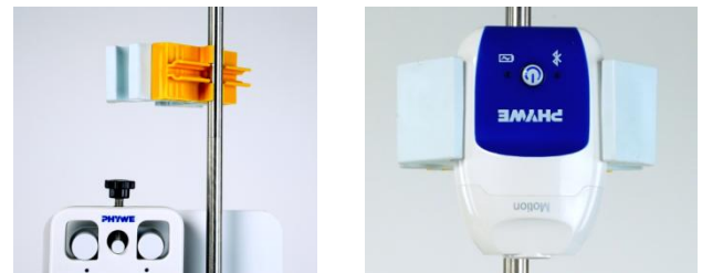
Fig. 6+7 Mounting the motion sensor
