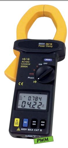
**VA6600** is a multifunctional and AC + DC true RMS clamp. A double screen shows two electrical quantities simultaneously: U and I , U and Hz , I and Hz , W and the power factor  $\cos\varphi$ , VA and VAR. The measurement of active, reactive and apparent power is possible in single-phase, three-phase three-wire or three-phase four-wire, on balanced or unbalanced load (using microprocessor calculations). The ratings are altered automatically.
