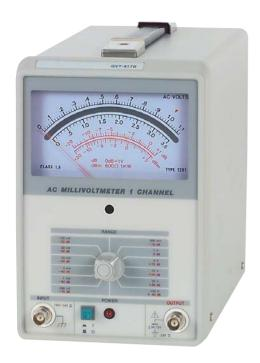
GVT417 is a millivoltmeter for the measuring of sinusoidal voltages from  $10\mu V$  to 100V, in the 10~Hz to 1MHz band. The dial is graduated in volts and dB for the direct measurement of amplifier increases.
