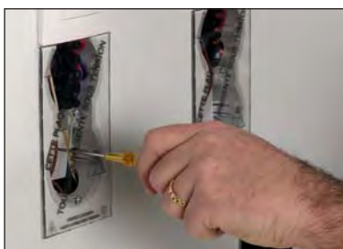
Coupling a receiver + transmitter pair through the protection window by pressing a contact.
