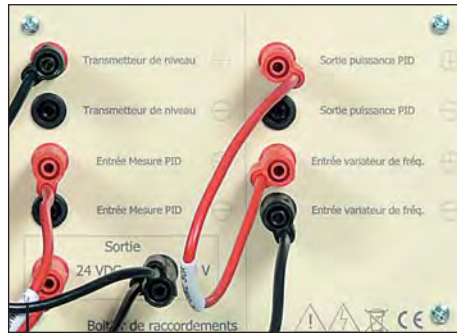
Terminal block with inputs and outputs of variator control and PID sensors
