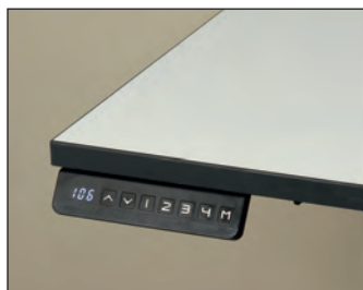
Electric command affixed under the worktop. 4 memorized positions. Digital height display. Manual controls with 3mm steps.
