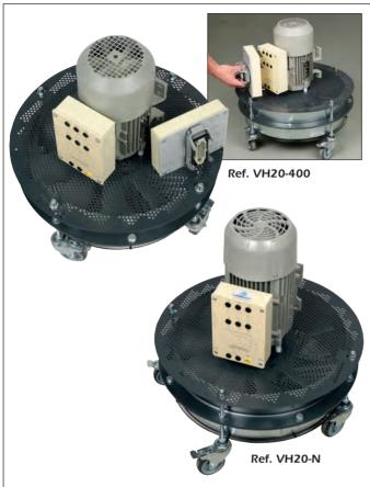
On the base of a propeller fan, a 1500W motor is direct-coupled to the propeller in a 500mm diameter shaft. In this way, this small group forms a dynamic load designed for studying the load currents of a motor.
