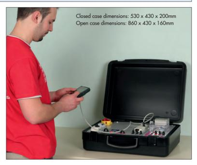
VAL-VAR is a study case for the speed controller ATV32 for asynchronous machine. It contains all the equipment required for autonomous operation.
