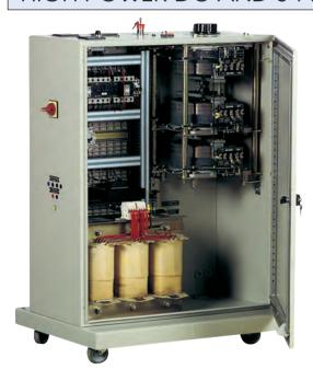
This power supply, which is varied using an autotransformer, can be networked so that it can power other stations. The DC outputs are insulated from the mains, as stipulated in the standard, and monitored by a continuous insulation monitoring device for the safety of users. This monitoring allows the DC output to be networked. The transformer complies with the NFEN6158 norm.
