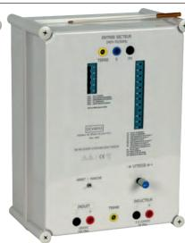
DCVAR2 and DCVAR43 speed controllers control separately excited or permanent magnet DC motors. On the front, the RUN button powers up the speed controller and the potentiometer varies the speed of rotation of the motor.
