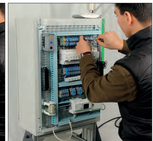
Grid support at the back of the box allowing the wiring of the grid before it is used in the cabinet.
