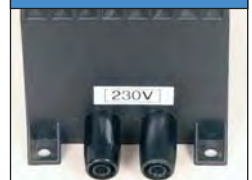
PRIMARY 230V ON MAINS CABLE
